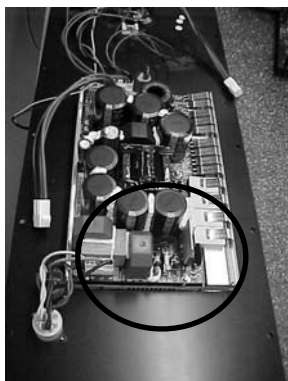
Fig.24. Fuse placement
