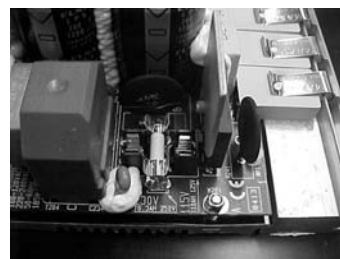
Fig.25. Fuse position (front view):
